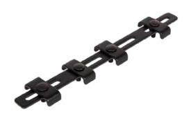
The Bar Splice Kit provides additional strength when joining two basket trays on a horizontal plane. Each kit includes one straight bar splice and 4 sets of M6x20 carriage bolts, M6 nuts, and top splice washers.
