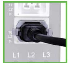
The IEX Lock-VP bezel inserts into the outlet to provide a secure, locking connection for both standard and V-LOCK C14 plugs.
