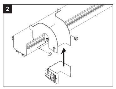
• Slide the cover onto the Side Drop.
