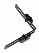
This kit provides support at horizontal 90 degree turns and tee junctions. Each kit includes one right-angle bar splice and two sets of M6x20 carriage bolts, M6 nuts, and top splice washers.
