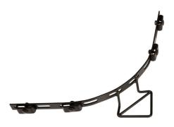
Radius Splices are a fast and easy solution for maintaining minimum cable bend radius at 90 degree bends, tees, and cross intersections. Each kit includes one radius bar and four sets of M6x20 carriage bolts, M6 nuts, and top splice washers.
